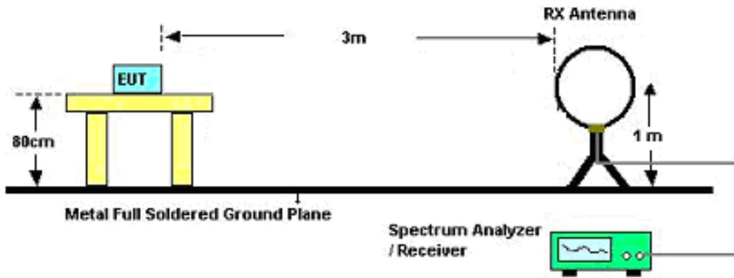
For Radiated Emissions: 30MHz~1GHz
