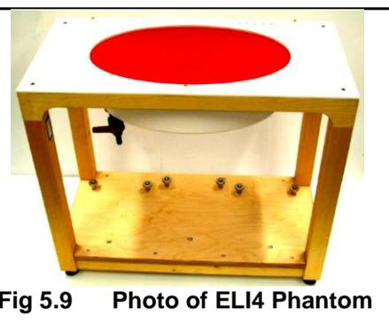
The ELI4 phantom is intended for compliance testing of handheld and body-mounted wireless devices in the frequency range of 30 MHz to 6 GHz. ELI4 is fully compatible with standard and all known tissue simulating liquids.
