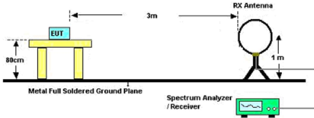
For Radiated Emissions: 30MHz~1GHz
