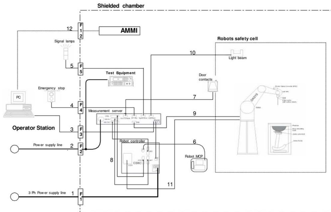
The DASYS5 system for performing compliance tests consist of the following items:
