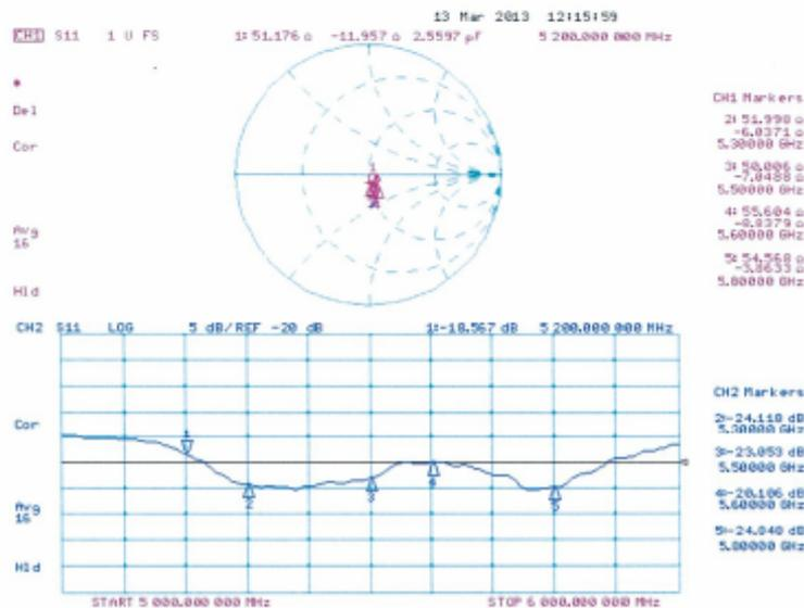
**Impedance Measurement Plot for Body TSL (UL Spacer #1)**
