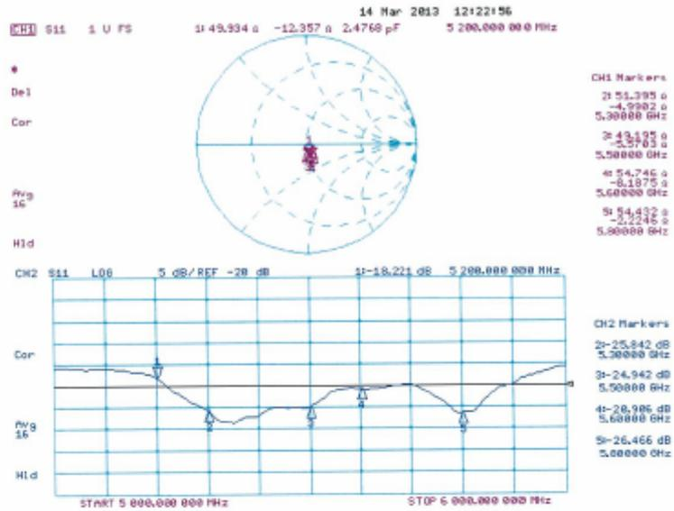
**Impedance Measurement Plot for Body TSL (UL Spacer #2)**
