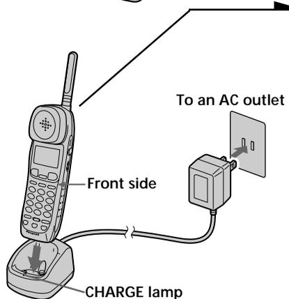
**4** Connect the AC power adaptor to an AC outlet and place the cordless handset on the charger. The CHARGE lamp on the charger lights up when the cordless handset is properly seated on the charge terminals of the charger. Charge the battery pack for more than 12 hours so that the battery is fully charged. The CHARGE lamp remains lit even after charging is completed.
