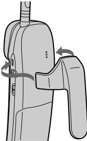
Press the belt clip to the cordless handset. Make sure that the side tabs click and go into the holes on the sides of the cordless handset.
