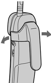
While pressing the back of the belt clip, pull the sides one by one until the tabs come off from the holes.
