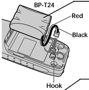
**2** Connect the battery connector with correct polarity (black wire goes on lower side and red wire goes on upper side).
