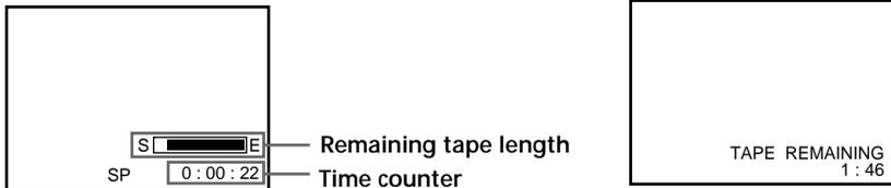
To check the remaining tape length of a T-140 or T-180 tape, set TAPE SELECT in the ADVANCED OPTIONS menu to 180. (For details, see page35.)
