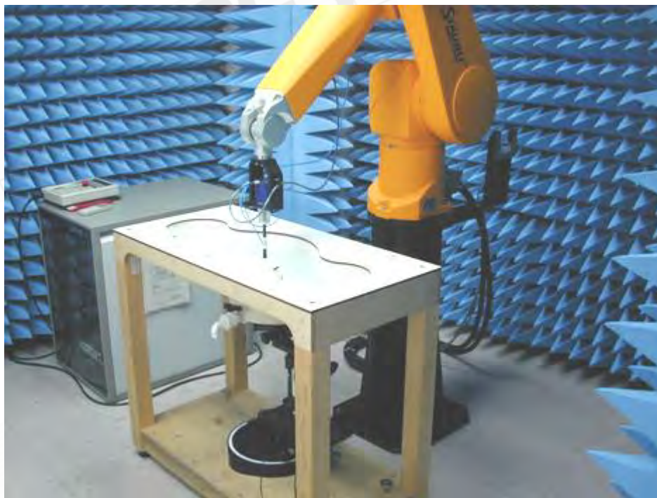
Fig.1 Photograph of the SAR measurement System
