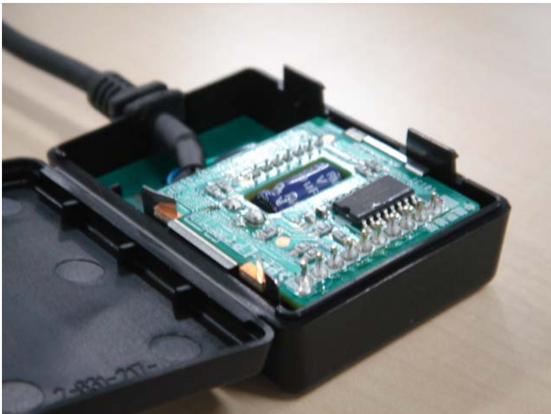
Transmitter Module cover opened 2
