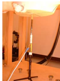
2450MHz System performance check setup
