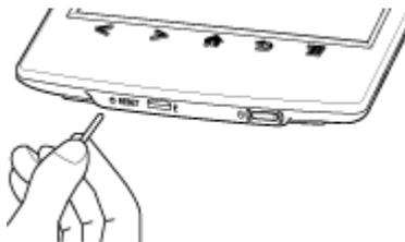
Press the RESET button with a small pin or clip.
