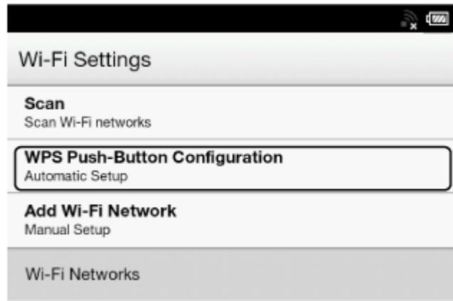
2. On your Wi-Fi router, press the “WPS” or “Connect” button within 2 minutes.\* The Reader automatically attempts to establish a Wi-Fi connection.
