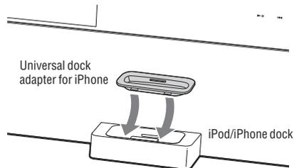
To remove the universal dock adapter for iPhone, pull it up with your fingernail or a flat object using the slot inside the adapter.
