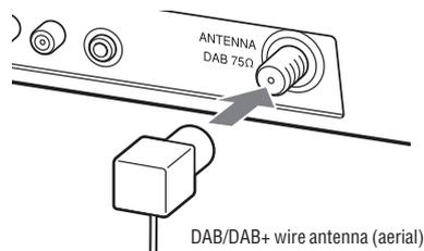
Use an external DAB/DAB+ antenna for a more robust DAB/DAB+ signal. It is recommended you only use the supplied DAB/DAB+ wire antenna for areas of strong DAB/DAB+ reception or as a temporary measure until you install an optional external antenna.
