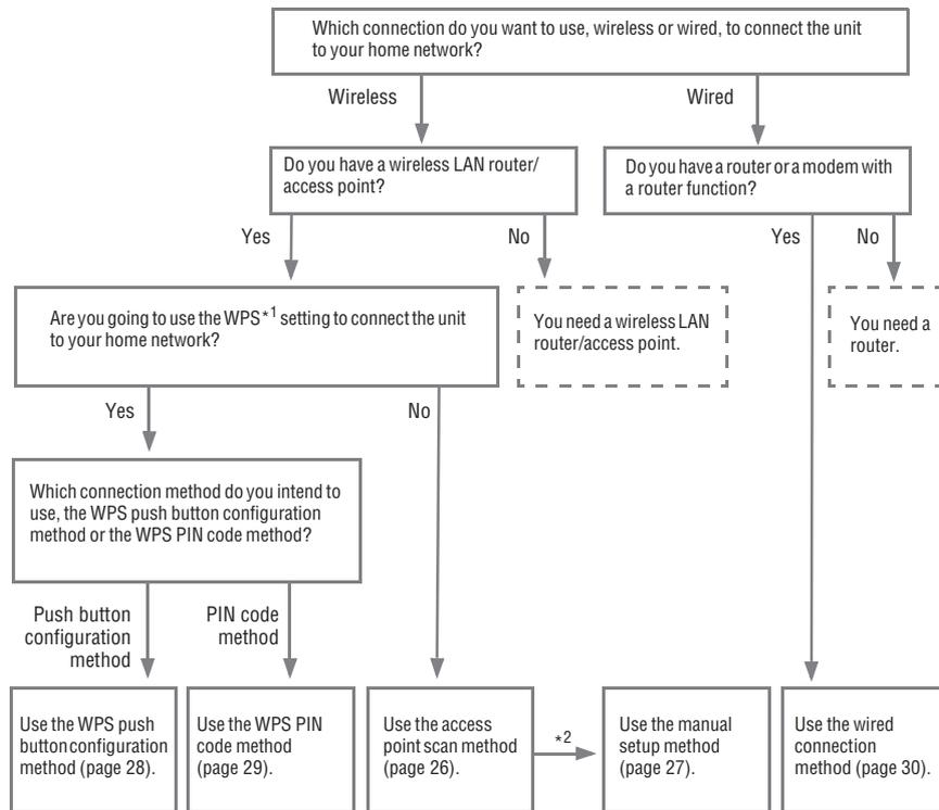
\*1 WPS (Wi-Fi Protected Setup) is a standard created by the Wi-Fi Alliance allowing you to setup a wireless network easily and securely.
