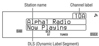
Press DISPLAY repeatedly to view information such as ensemble label or frequency of the current station. Press BACK to return to the service component list.
