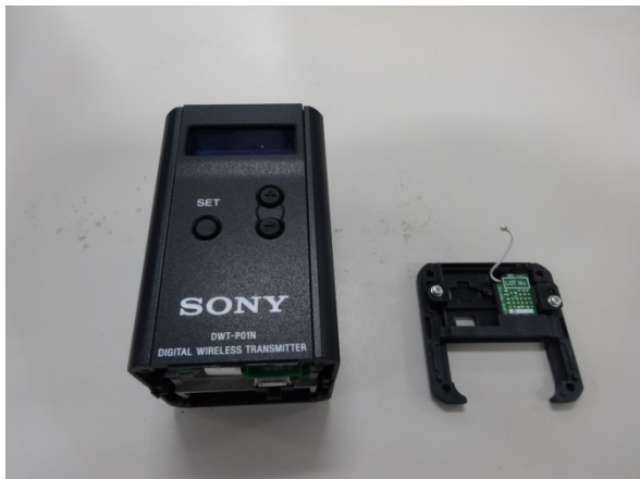
Fig.03 Detach Lower Panel
