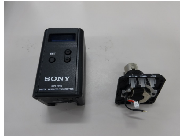
Fig.02 Detach Upper Parts
