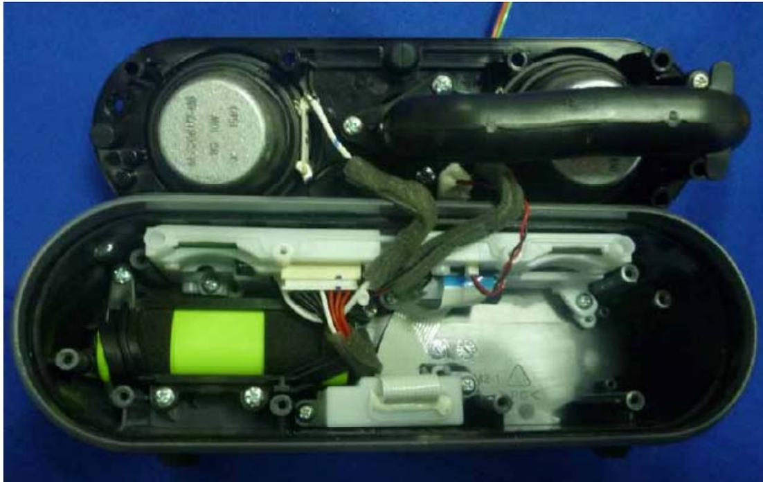
2d: Install the speaker holder with screws, then install the speaker grill.
