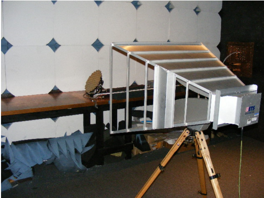
Figure G-11 – Radiated Spurious Emissions Test Setup, 200 MHz – 1 GHz
