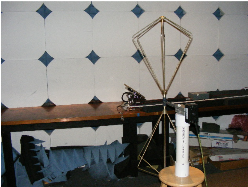
Figure G-10 – Radiated Spurious Emissions Test Setup, 25 MHz – 200 MHz
