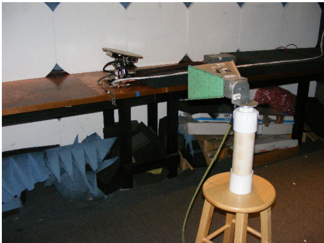
Figure G-12 – Radiated Spurious Emissions Test Setup, 1 GHz – 18 GHz
