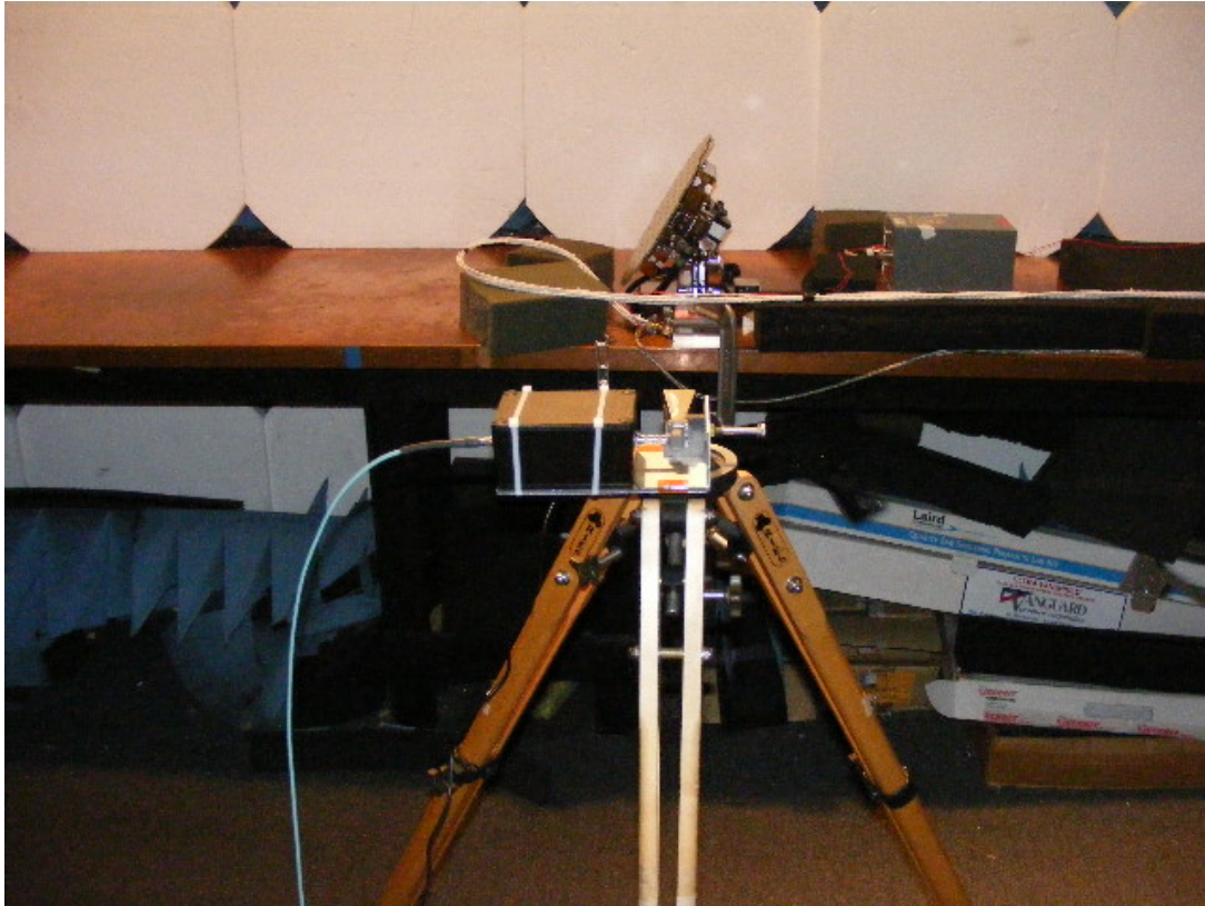
Figure G-13 – Radiated Spurious Emissions Test Setup, 18 GHz – 40 GHz
