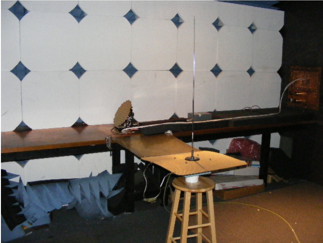
Figure G-9 – Radiated Spurious Emissions Test Setup, 2 MHz – 25 MHz
