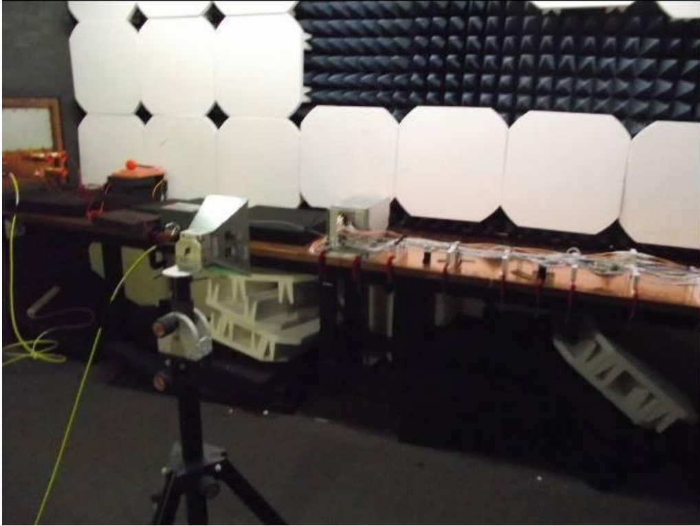
Figure G-15 – Radiated Spurious Emissions Test Setup, 1 GHz – 10.3 GHz, Horizontal Polarization
