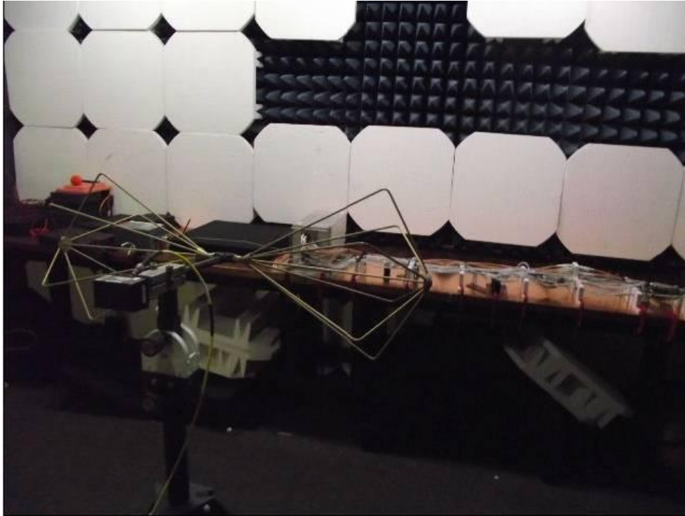
Figure G-11 – Radiated Spurious Emissions Test Setup, 25 MHz – 200 MHz, Horizontal Polarization
