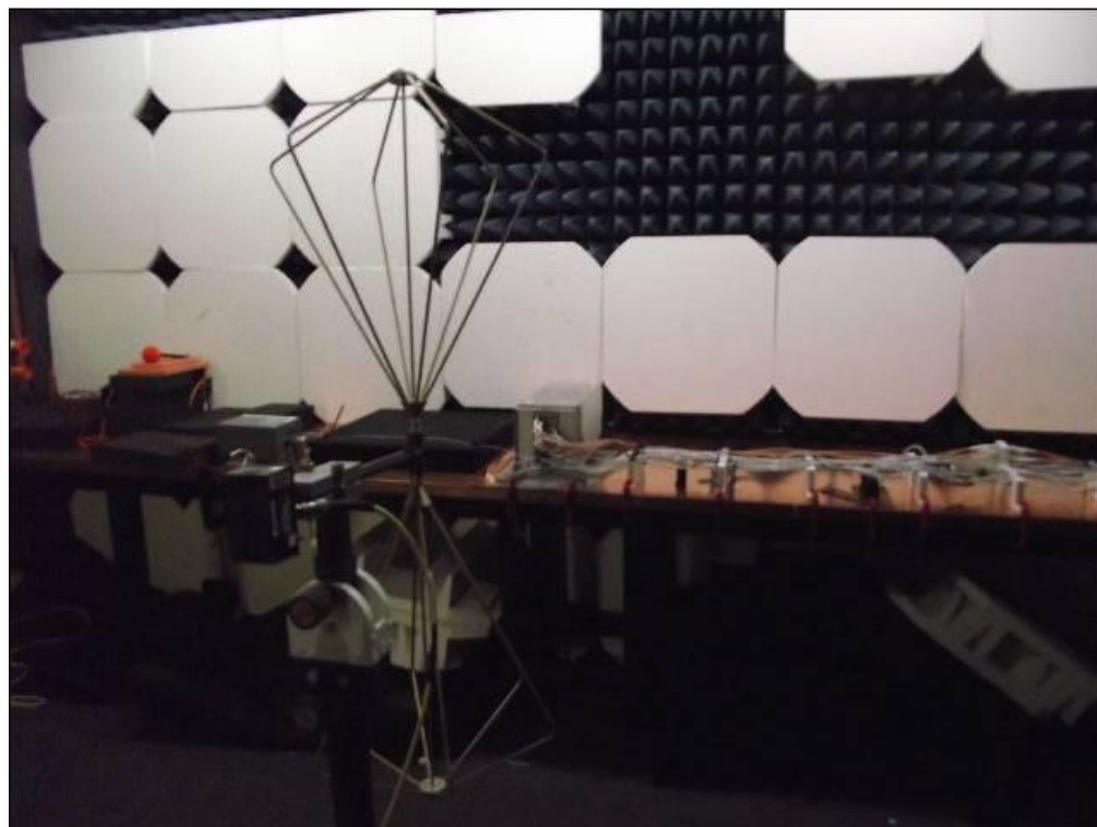
Figure G-10 – Radiated Spurious Emissions Test Setup, 25 MHz – 200 MHz, Vertical Polarization
