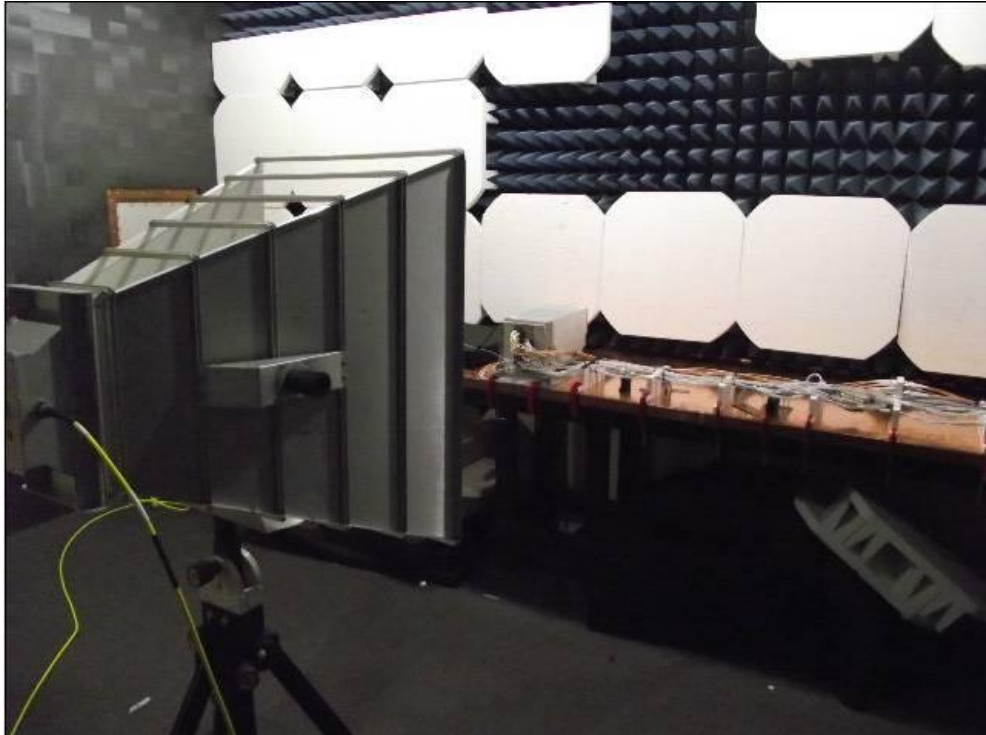
Figure G-13 – Radiated Spurious Emissions Test Setup, 200 MHz – 1 GHz, Horizontal Polarization
