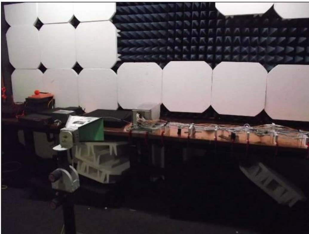
Figure G-14 – Radiated Spurious Emissions Test Setup, 1 GHz – 10.3 GHz, Vertical Polarization
