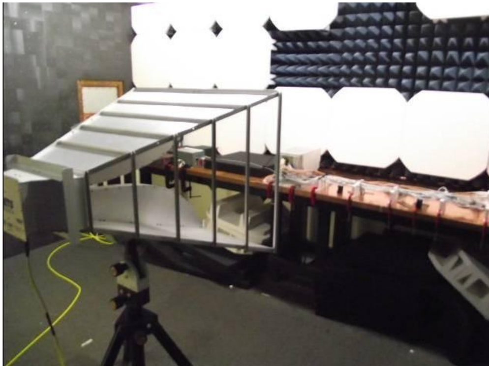
Figure G-12 – Radiated Spurious Emissions Test Setup, 200 MHz – 1 GHz, Vertical Polarization
