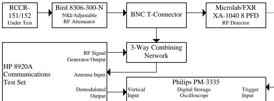
3. The HP 8920A Receiver was set to measure FM deviation with the audio bandwidth set at DC to greater than 15 kHz with the RF frequency set to 164.025 MHz. The attenuator was set for 40 dB.
