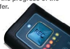
**7** After the computer has finished analyzing the lung sound, the lung score will be transmitted back to the stethoscope and displayed on the body. The light that corresponds with the score will be illuminated.
