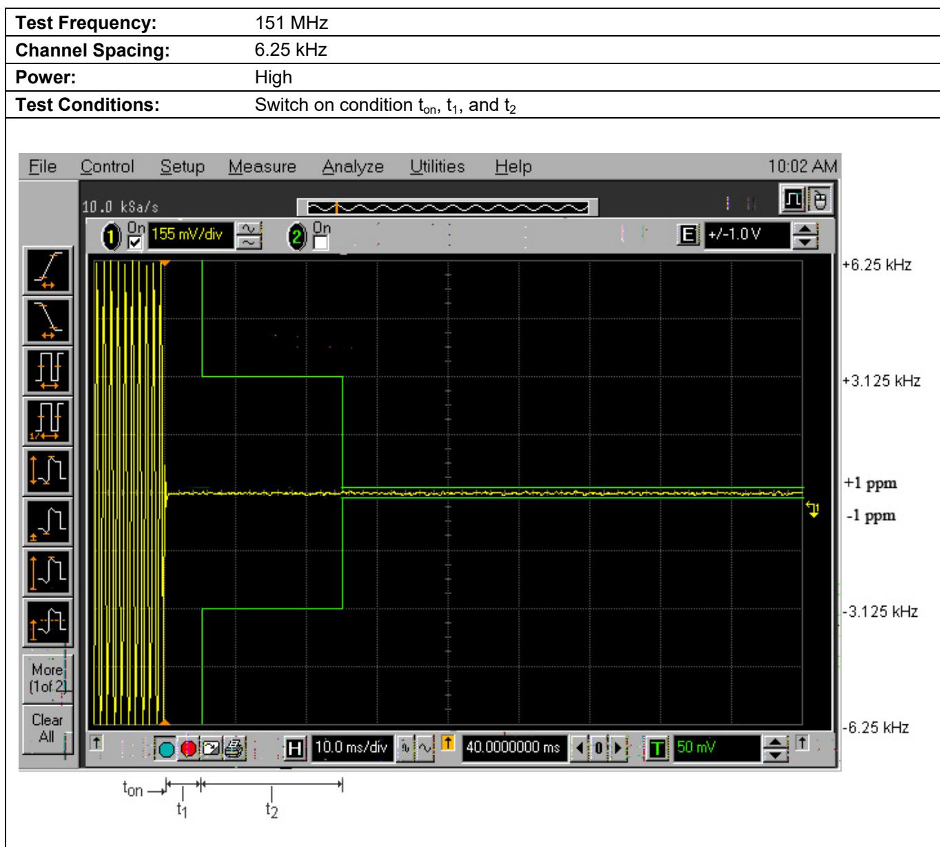
**Plot 5.12.3.6. Transient Frequency Behavior for 6.25 kHz Channel Spacing**
