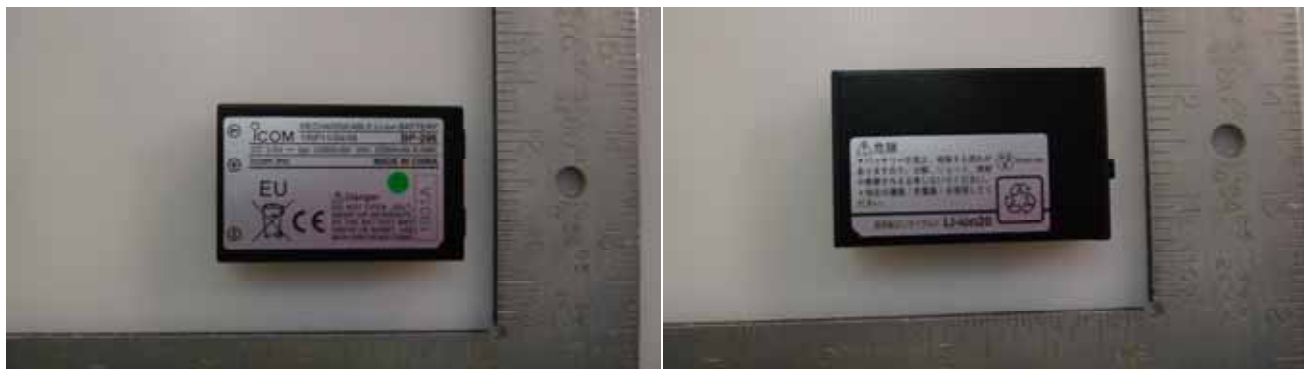
Li-ion Chargeable Battery (M/N: BP-296, 3.6V, 2350mAh)
