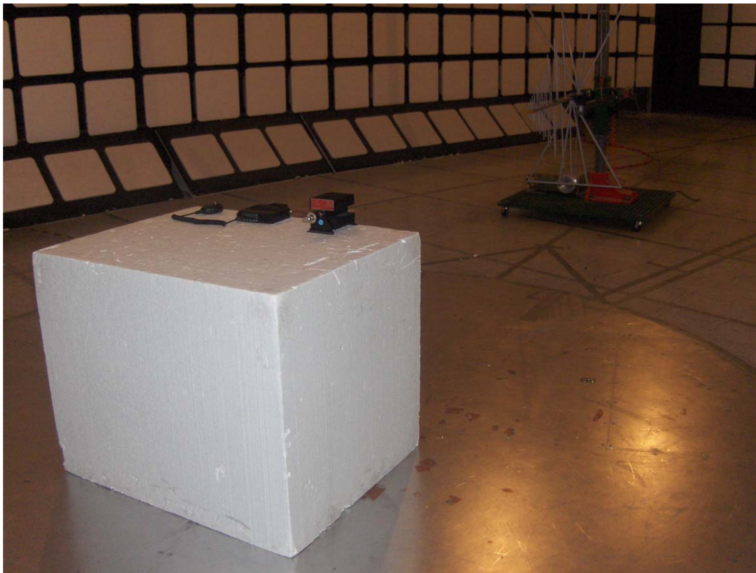
Plot #1: Radiated Emission Test Setup
