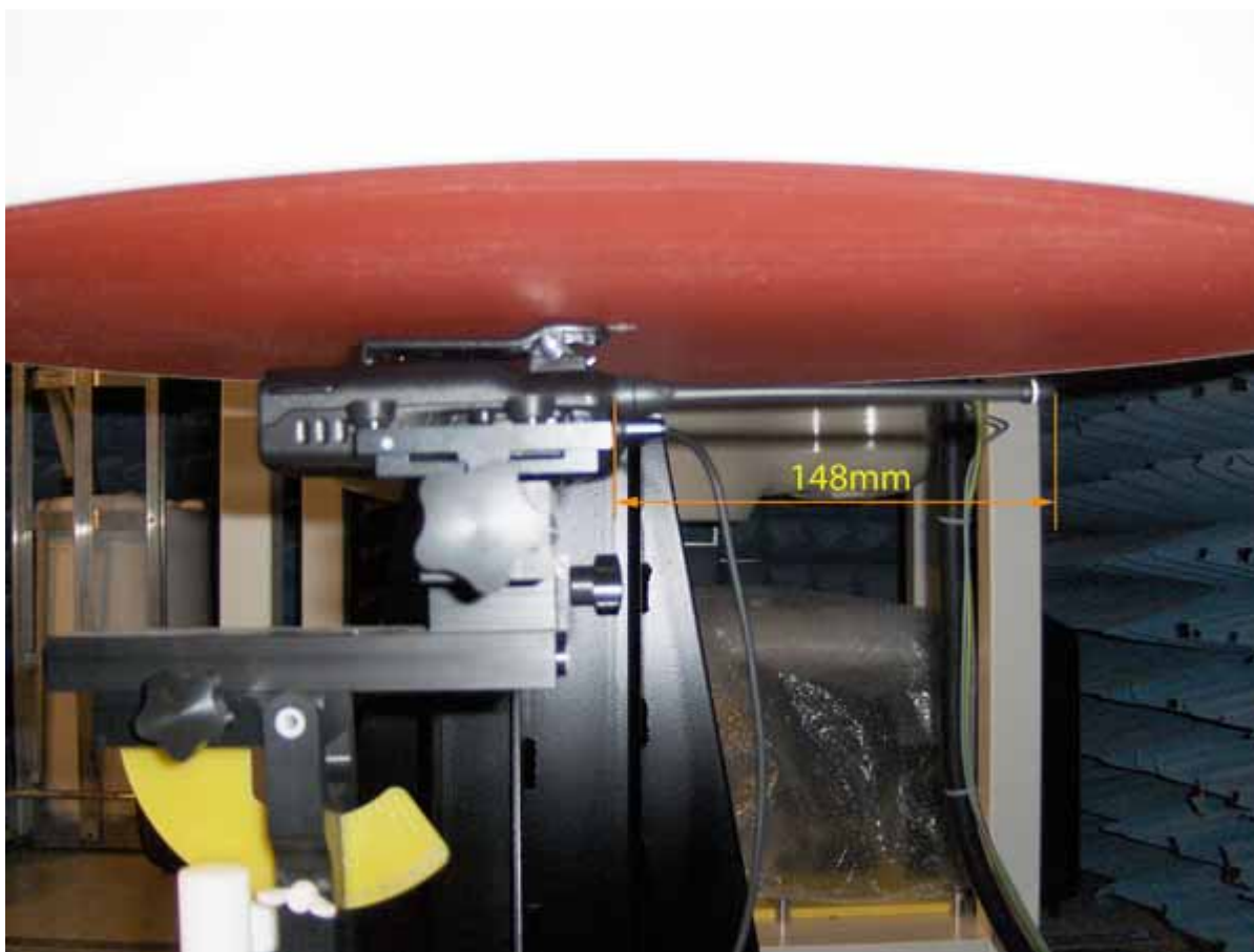
< FA-SC61UC cut antenna with the length of 148mm >
