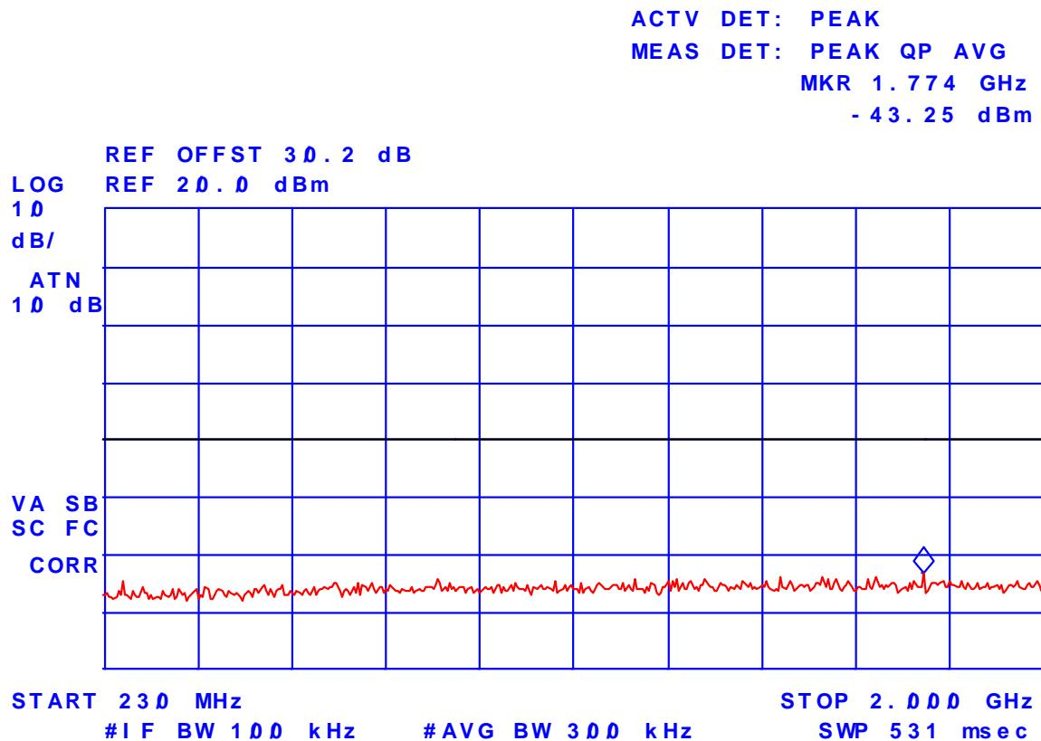
**Plot # 3: Transmitter Antenna Power Conducted Emissions**
