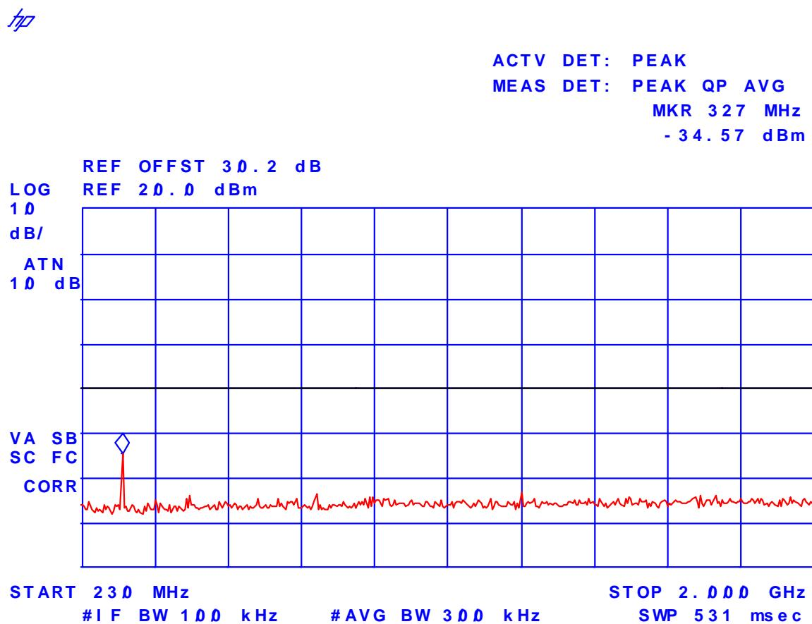
**Plot # 11: Transmitter Antenna Power Conducted Emissions**
