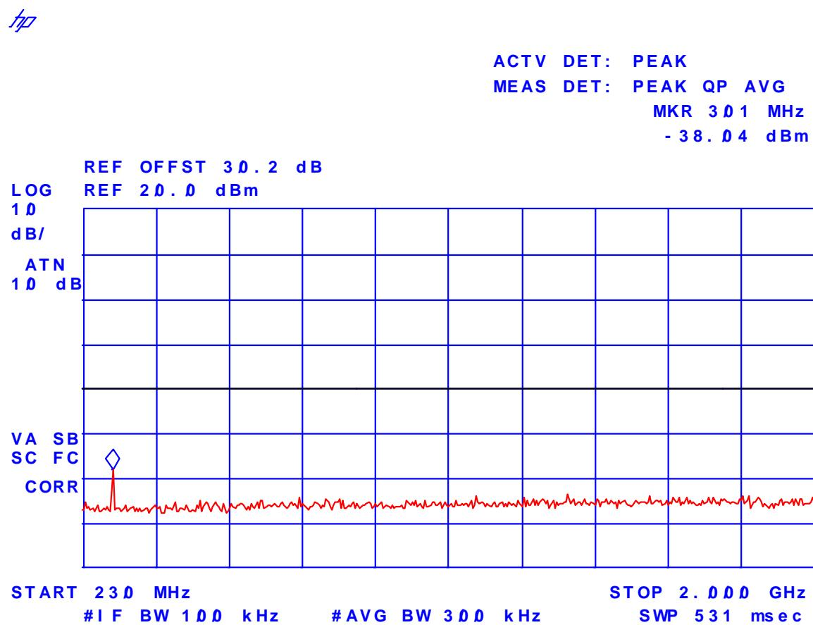
**Plot # 9: Transmitter Antenna Power Conducted Emissions**
