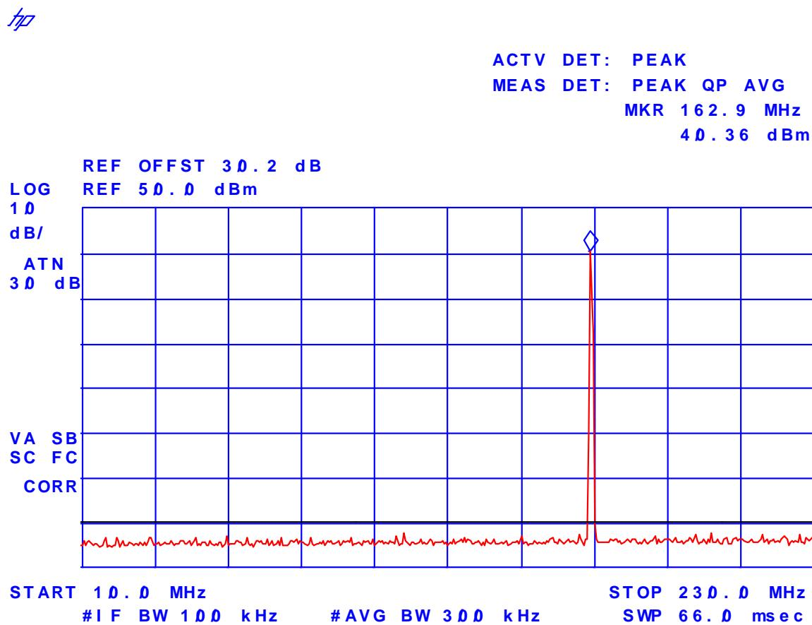
**Plot # 4: Transmitter Antenna Power Conducted Emissions**
