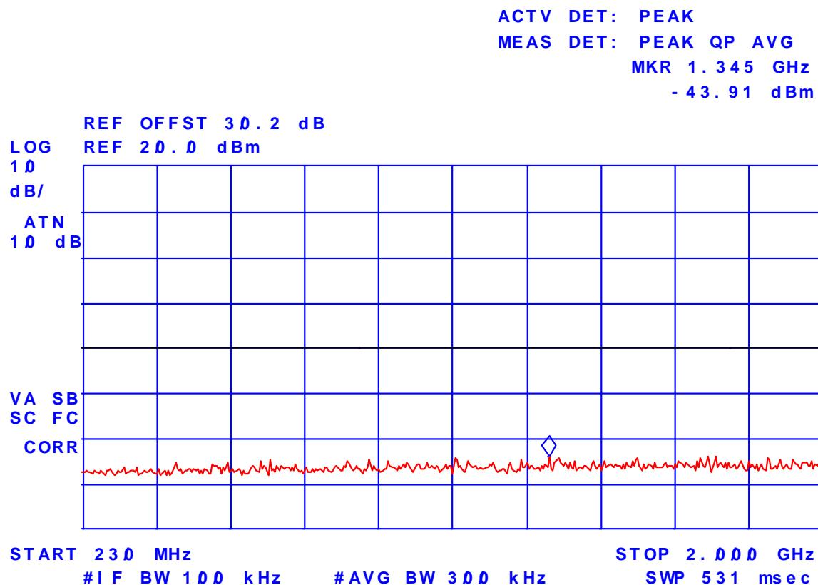
**Plot # 5: Transmitter Antenna Power Conducted Emissions**
