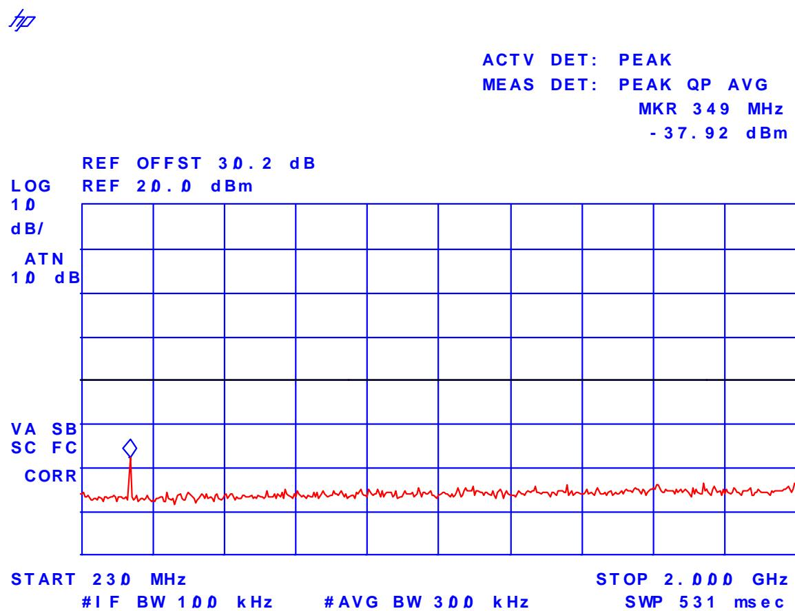
**Plot # 7: Transmitter Antenna Power Conducted Emissions**
