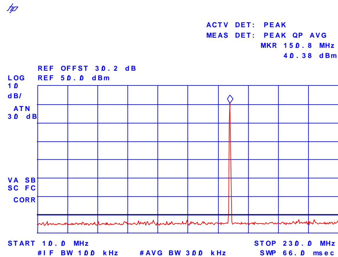
**Plot # 2: Transmitter Antenna Power Conducted Emissions**
