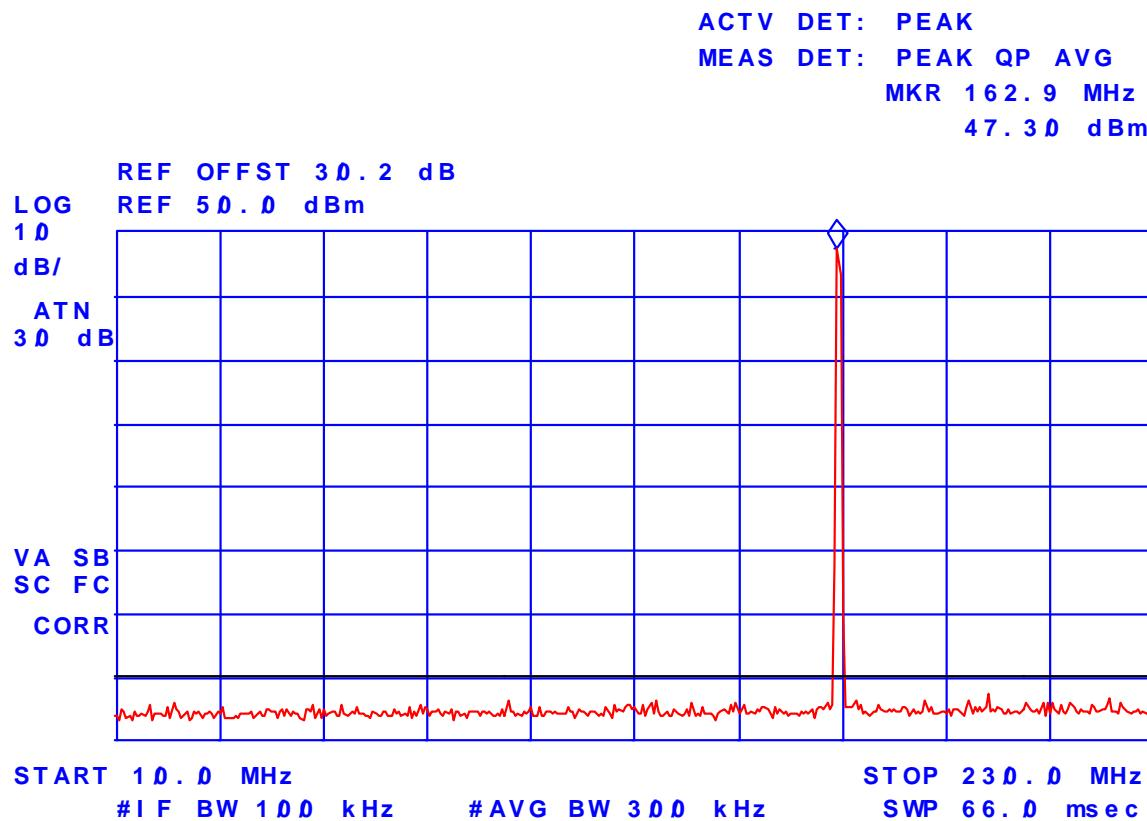
**Plot # 10: Transmitter Antenna Power Conducted Emissions**
