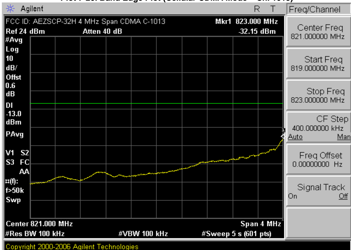
Plot 7-21. 4MHz Span Plot (Cellular CDMA Mode – Ch. 1013)
