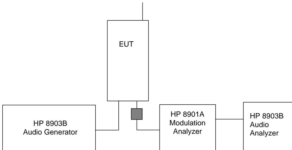
Fig. 3. Transmitter Audio Frequency & Tone Modulation Test Setup.
