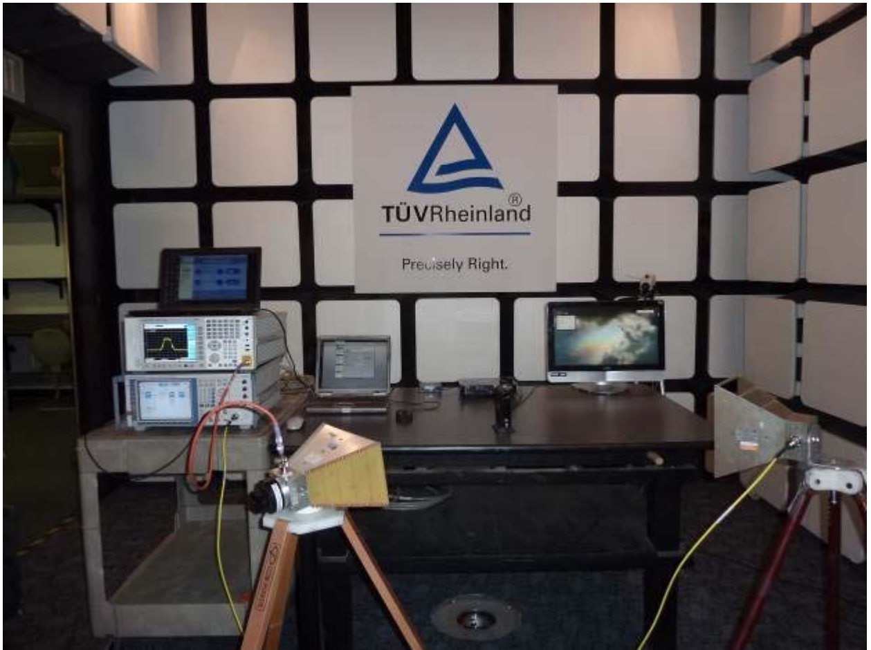
Figure 19: Dynamic Frequency Selection Test Setup – Front View
