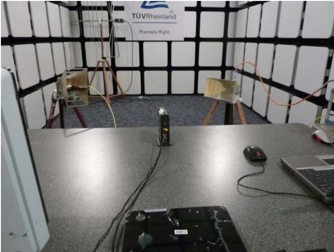
Figure 1: Dynamic Frequency Selection Test Setup – Rear View
