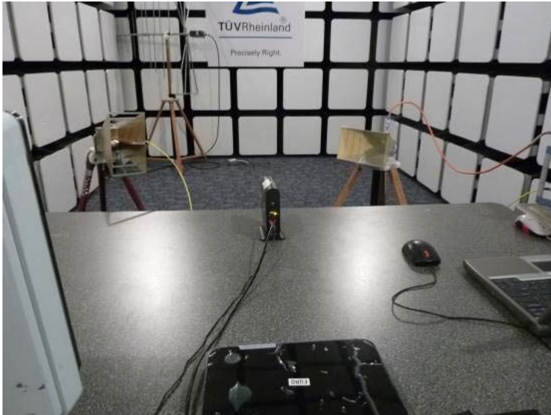
Figure 1: Dynamic Frequency Selection Test Setup – Rear View
