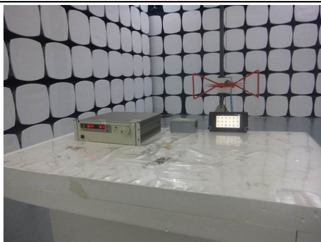
Radiated Spurious Emissions Test Setup Below 1GHz
