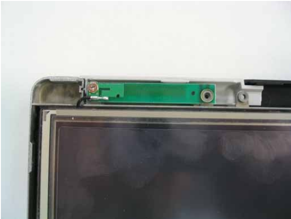
WLAN Main antenna magnified view
