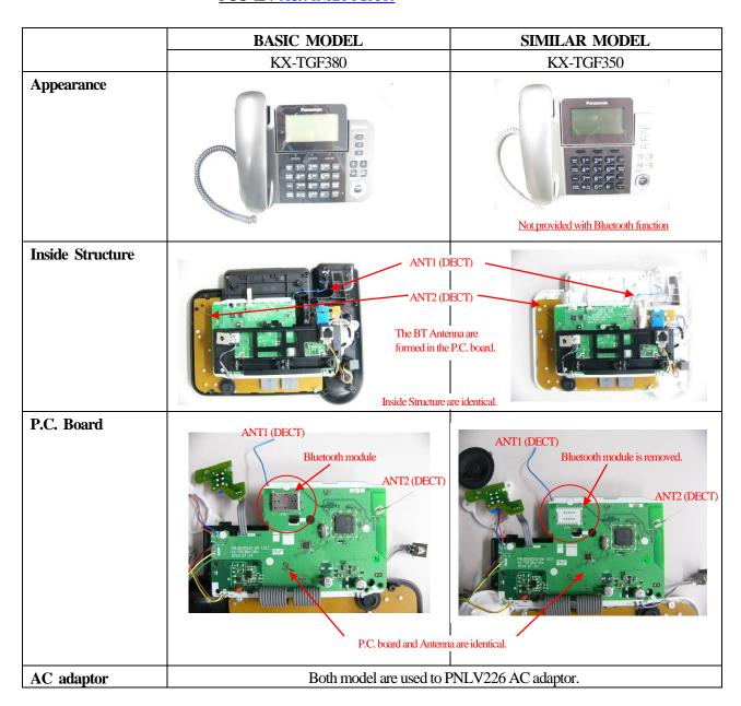
We declare that KX-TGF350 is used the another ID <u>ACJ96NKX-TGF350</u> because KX-TGF350 is not applied to FCC15 subpart C without 2.4GHz (Bluetooth) transmitter.
