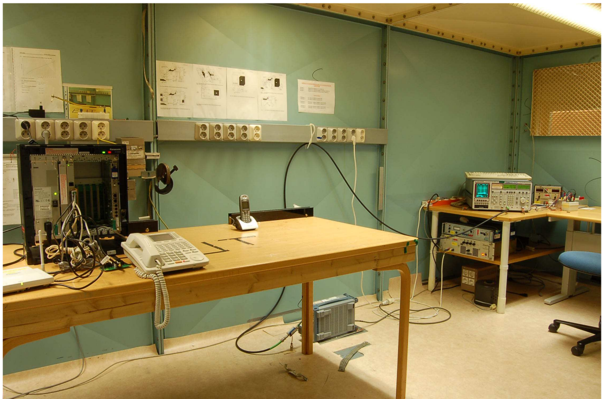
Power line Conducted Emissions Test
