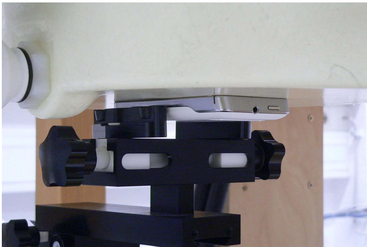
Fig. 22: Body worn configuration for KX-PRXA10, position 1, display towards the phantom, 0 mm distance.
