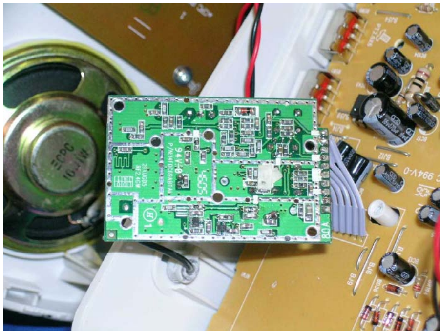
Base Unit Oscillator PCB solder side
