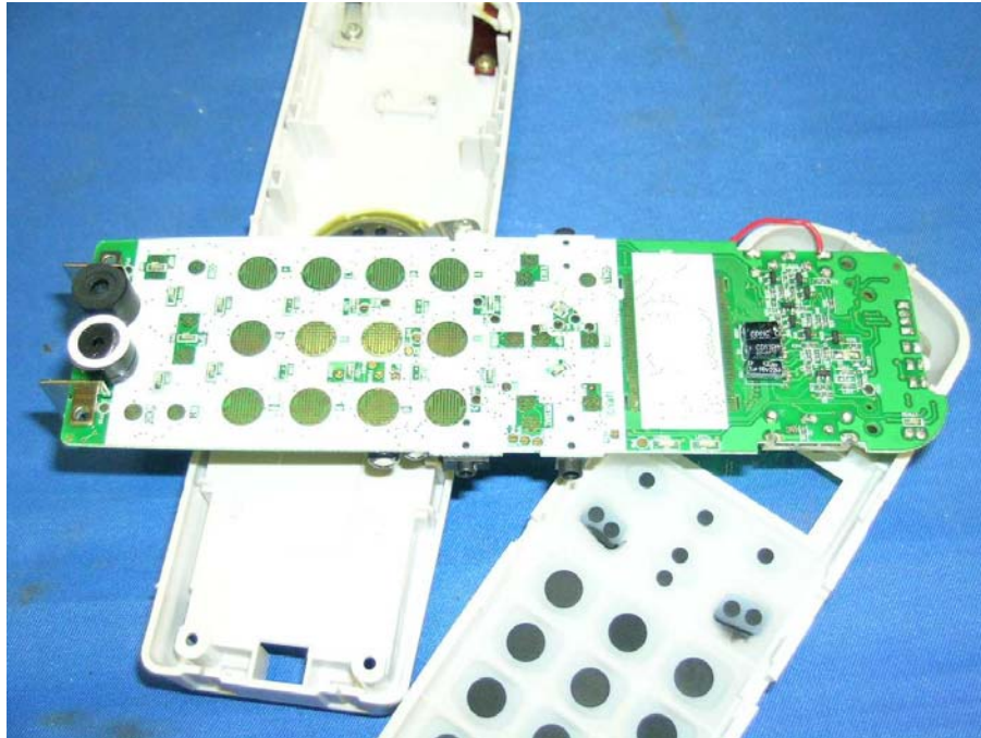
Handset Main PCB display side (View 2)
