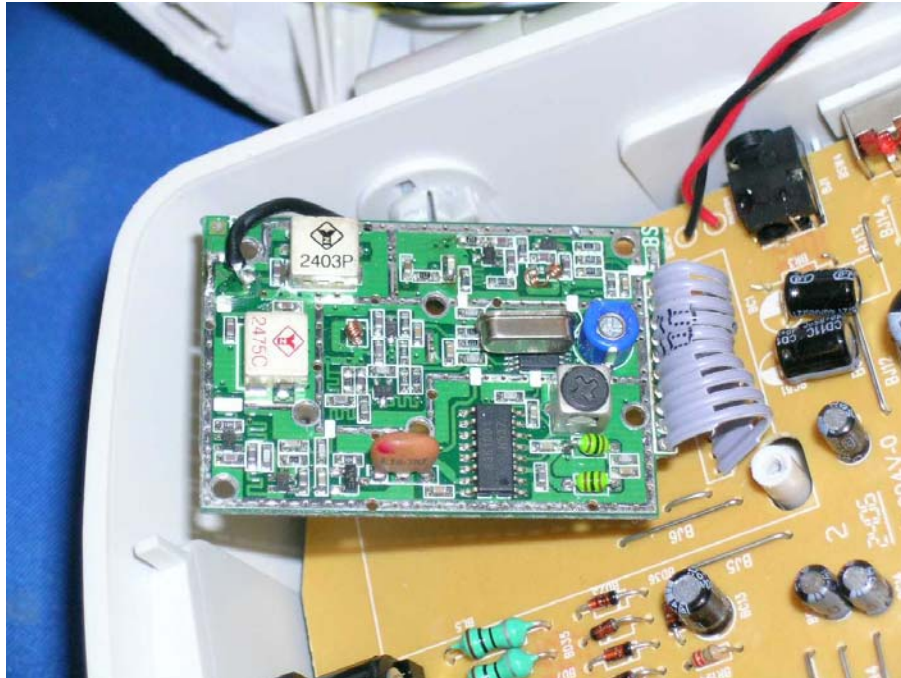
Base Unit Oscillator PCB comp side
