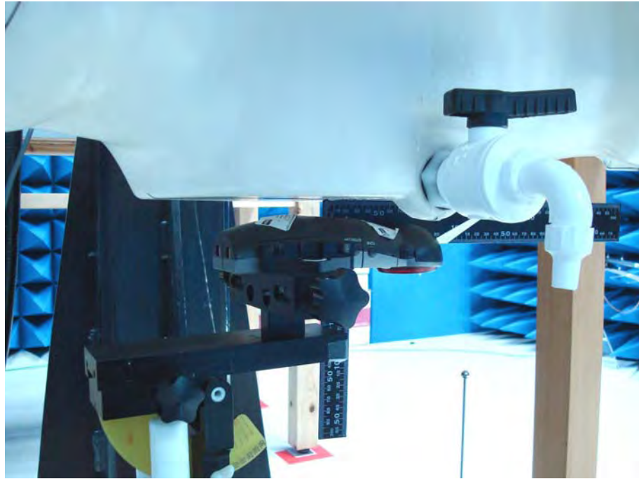
Figure 21. Body SAR Test Setup(Flat Section)_ 15mm space
