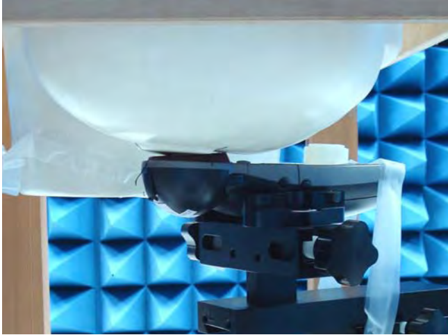
Figure 17. Right Head SAR Test Setup (Cheek)
