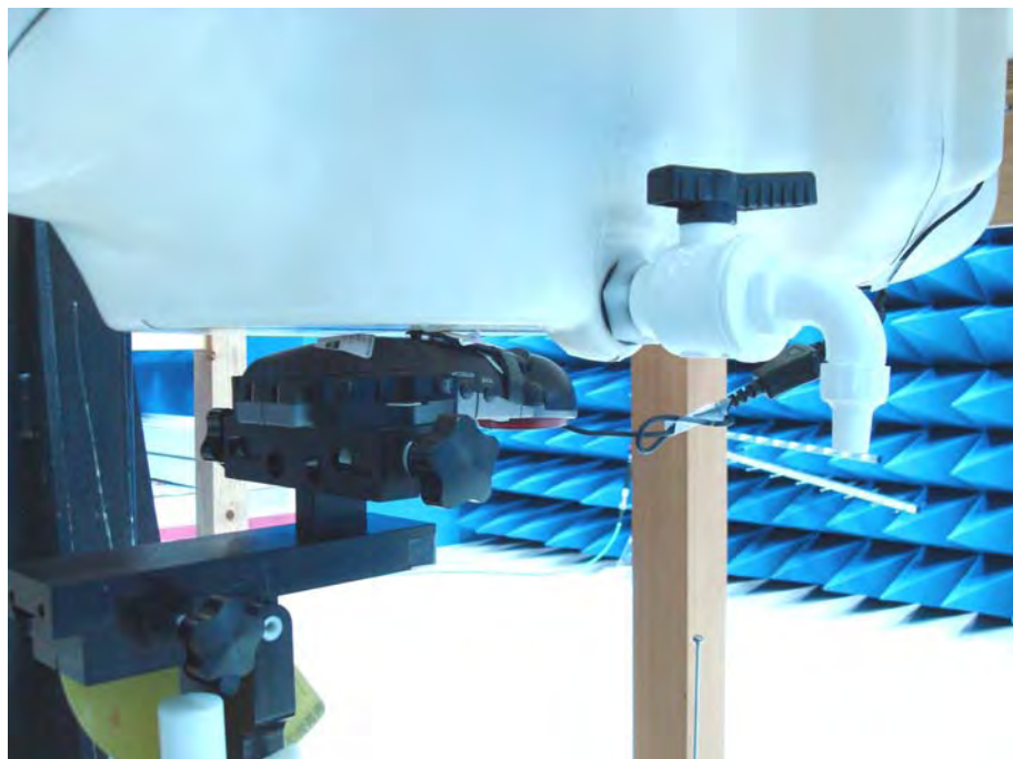
Figure 22. Body SAR Test Setup(Flat Section)_ Neck Loop
