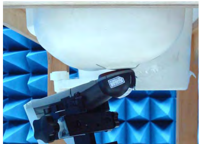
Figure 20. Left Head SAR Test Setup (Tilted)
