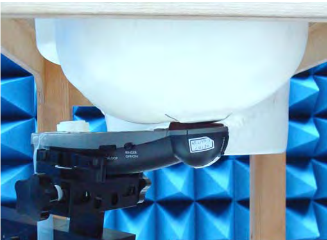
Figure 19. Left Head SAR Test Setup (Cheek)
