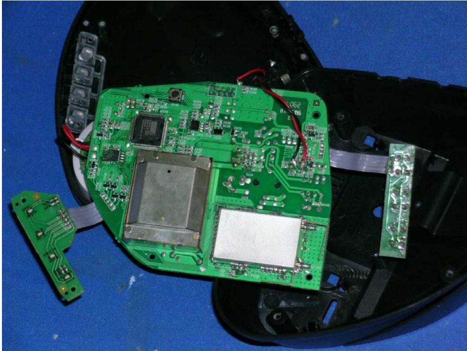
Base Unit Main PCB solder side (View 1)
