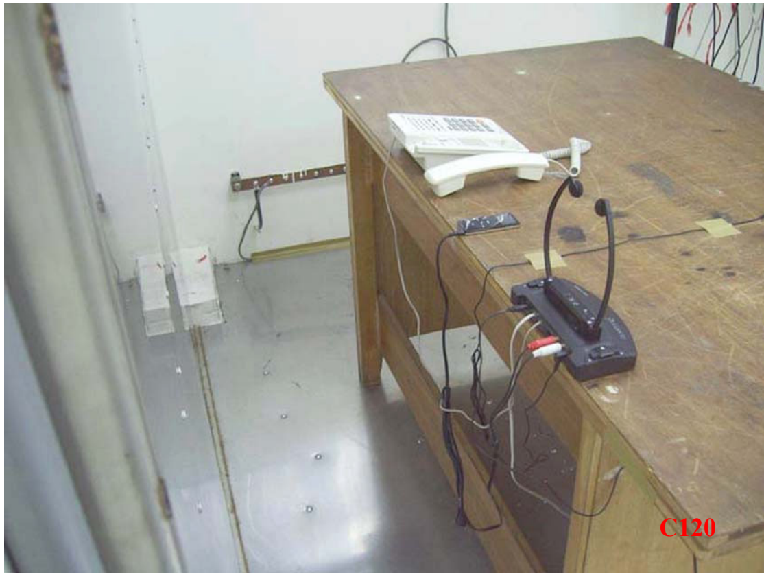
Photo 2: Conducted Emission Test Set-up photo
