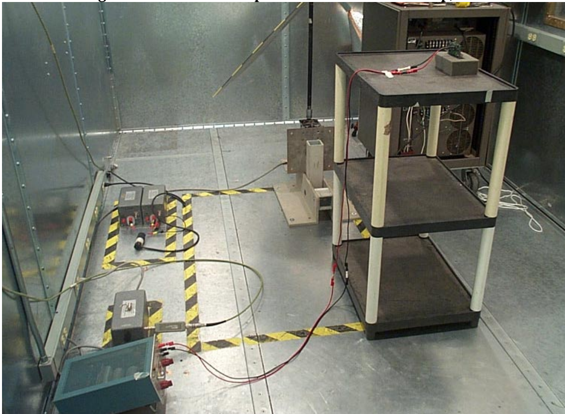
Figure C – 2 AC Conducted Emissions Test Setup
