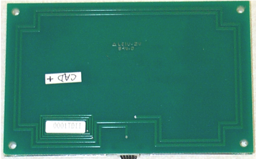
Figure 9.0-4 104 x 67 mm Antenna Board w/Ferrite
