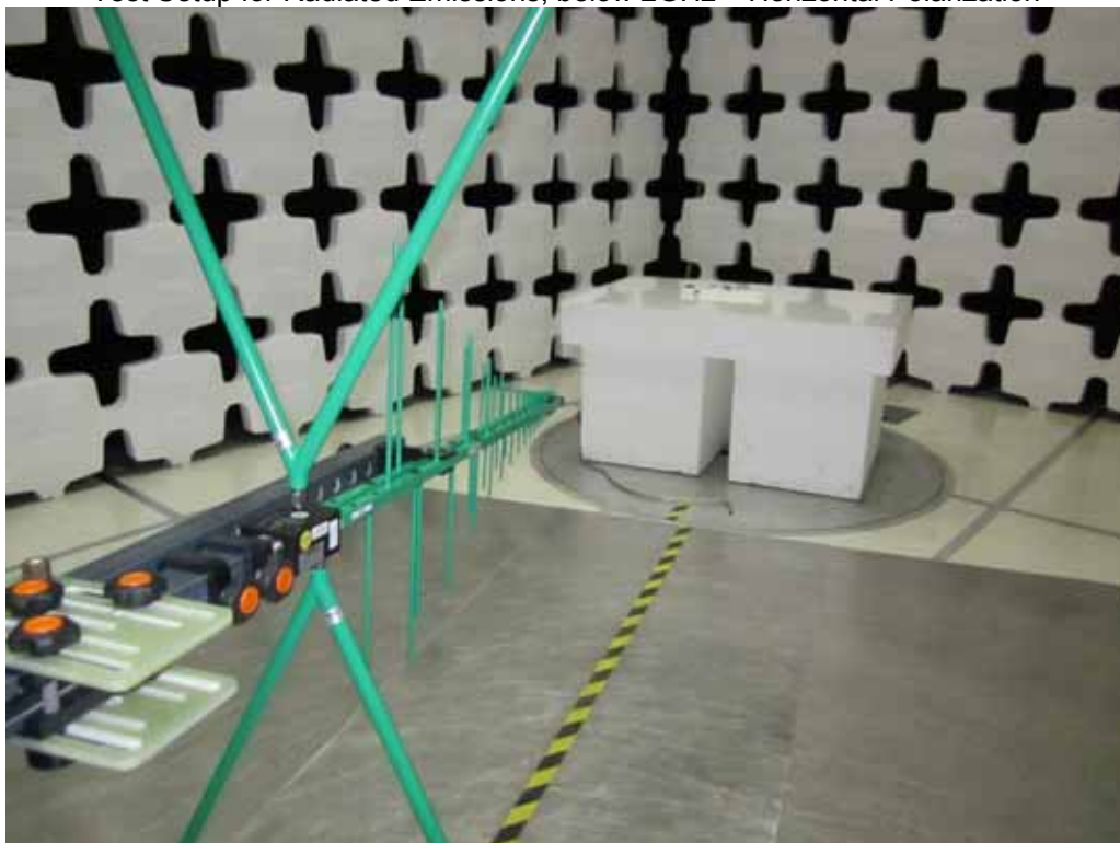
Test Setup for Radiated Emissions, below 2GHz – Vertical Polarization
