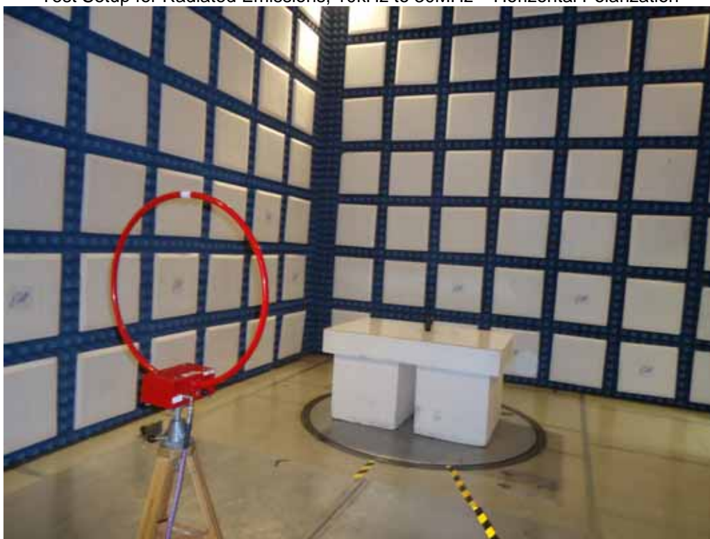
Test Setup for Radiated Emissions, 10kHz to 30MHz – Vertical Polarization
