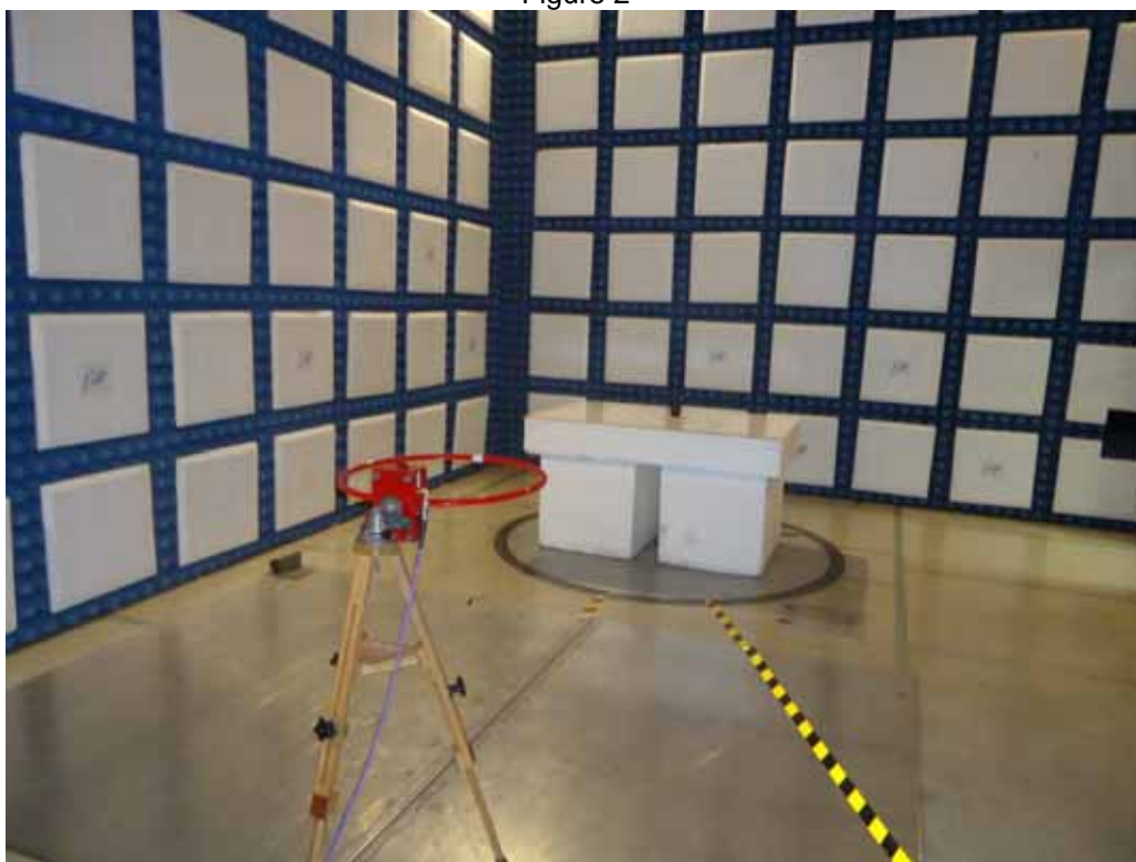
Test Setup for Radiated Emissions, 10kHz to 30MHz – Horizontal Polarization
