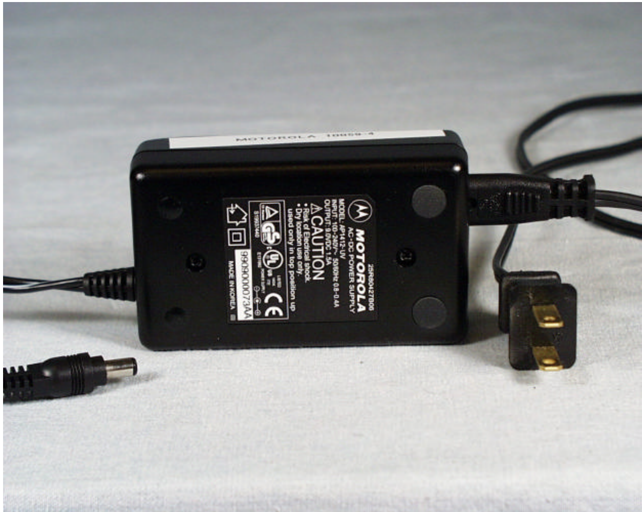
Base Station Power Supply
