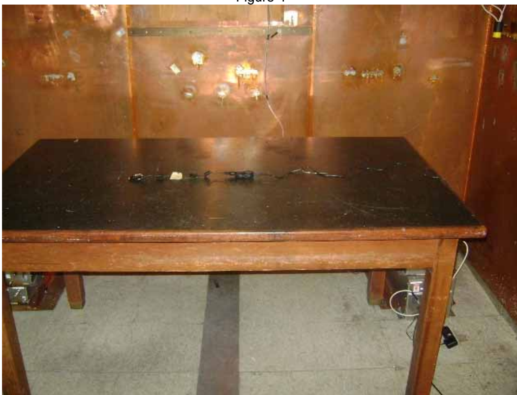
Test Setup for Conducted Emissions
