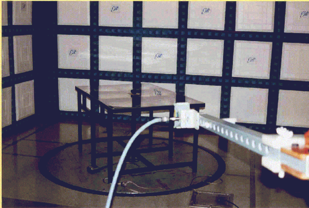
FIGURE 2A TEST SETUP FOR RADIATED EMISSIONS MEASUREMENTS MAXIMIZED FOR MEASUREMENT OF WORST CASE EMISSIONS VERTICAL POLARIZATION
