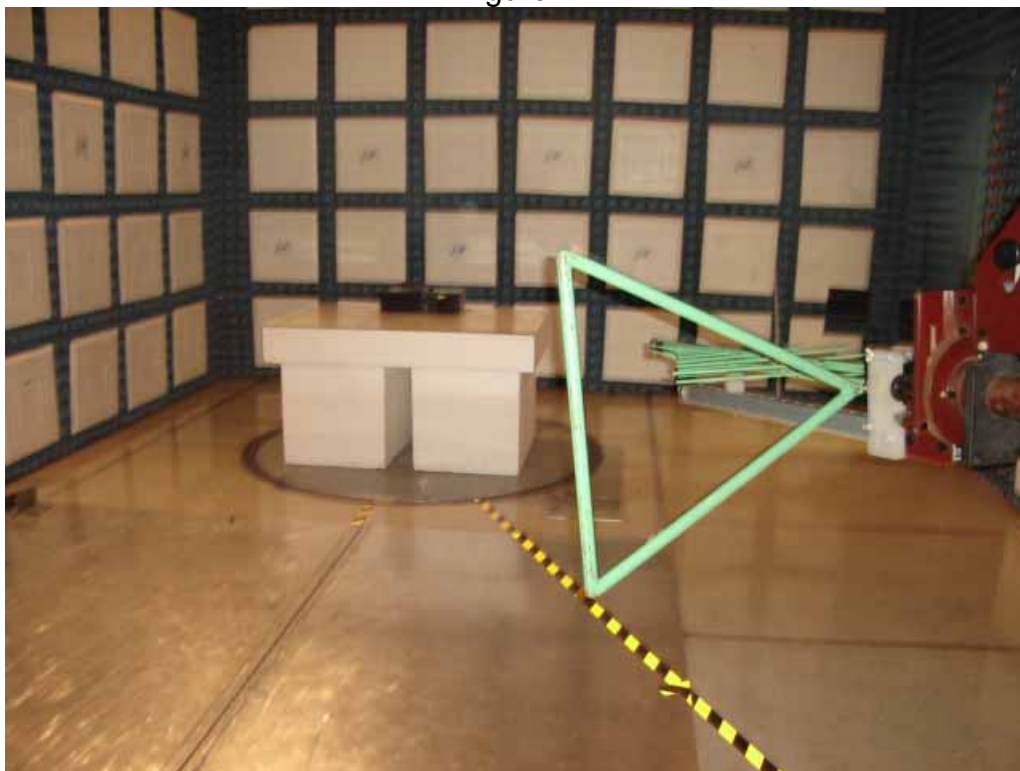
Test Item Set-up for Radiated Emissions Test – 30MHz to 1GHz Horizontal Polarity
