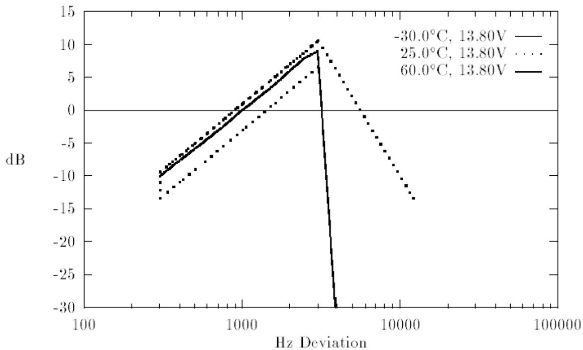
TRANSMIT AUDIO POST LIMITER LOW PASS FILTER RESPONSE
