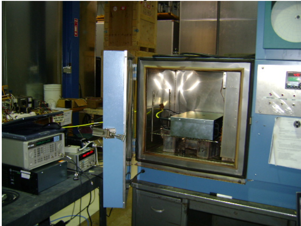
Test Set-up for Frequency Stability – Frequency vs. Temperature
