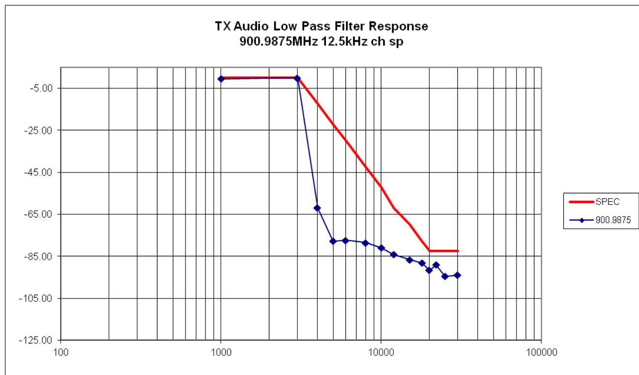
Figure 6C-5: 12.5 kHz Channel Spacing, 900.9875 MHz, Transmit Audio Low Pass Filter Response
