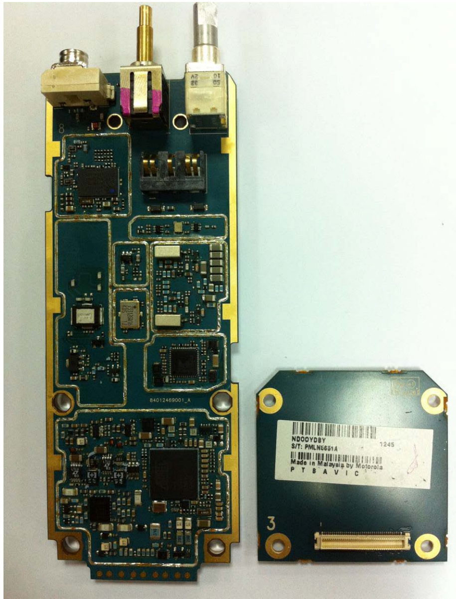
FIGURE 3- 4: NEO CSA WITH OPTION BOARD WITHOUT SHIELDS (BOTTOM SIDE)
