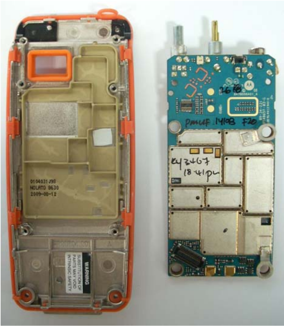
FIGURE 3-4: MOTOTRBO CHASIS, BOARD AND CAN SHIELDS
