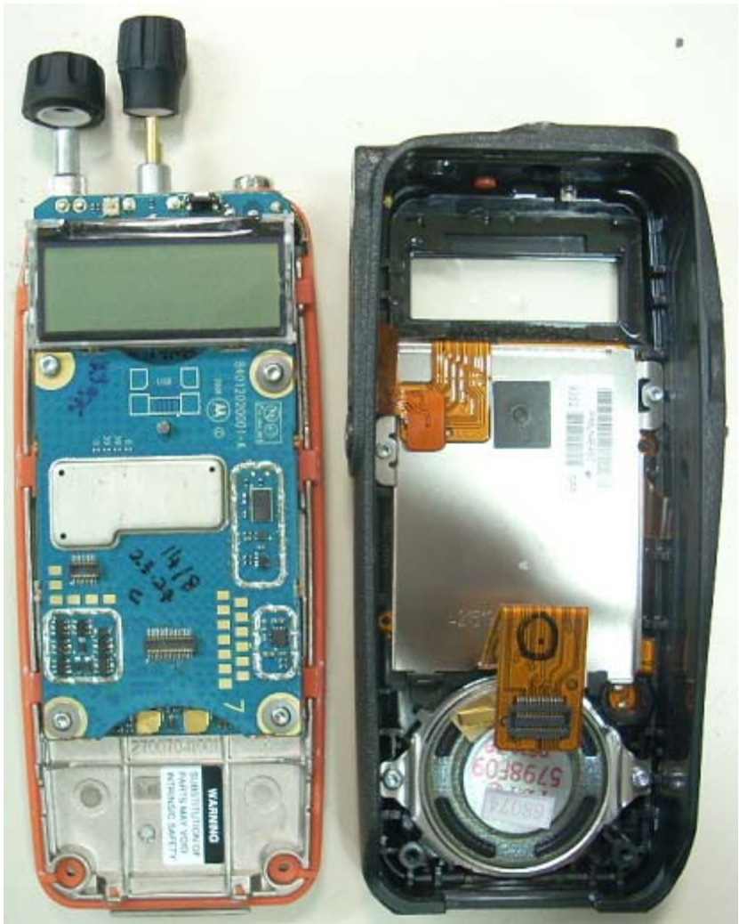
FIGURE 3- 1: MOTOTRBO COMPLETE INTERNAL OPEN UP VIEW.
