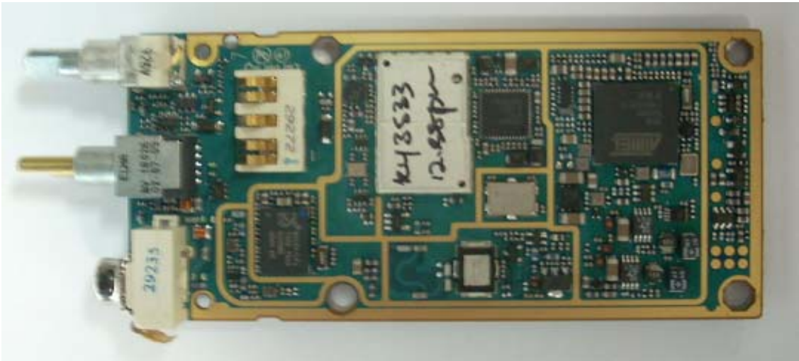
FIGURE 3-6: MOTOTRBO BOTTOM VIEW BOARD WITH GPS.
