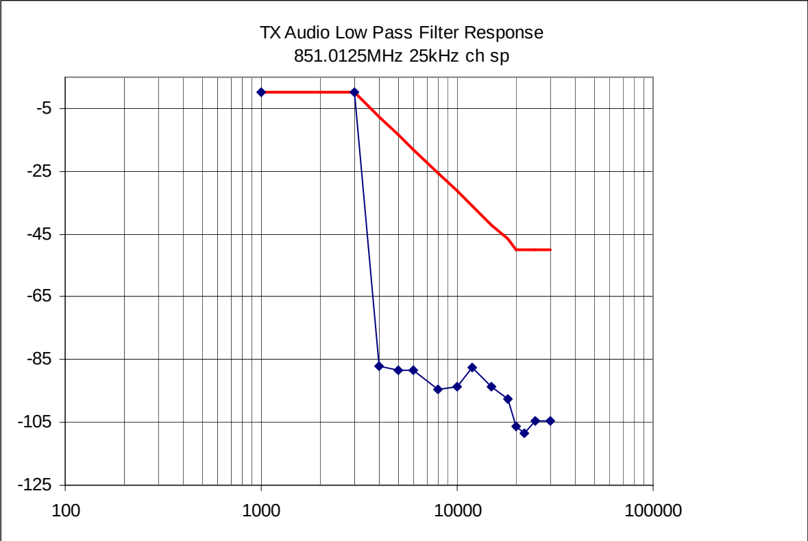
Figure 6C-2: 25 kHz Channel Spacing, 851.0125 MHz, Transmit Audio Low Pass Filter Response
